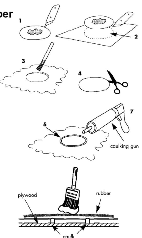
The above procedure results in a low profile. Seamless repair with identical weathering properties of original roof.
